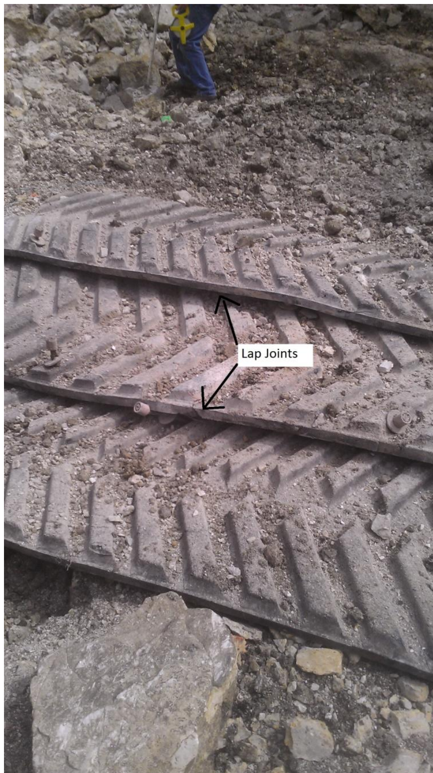
Figure 4.5 Tractor Tread Lap Joints
