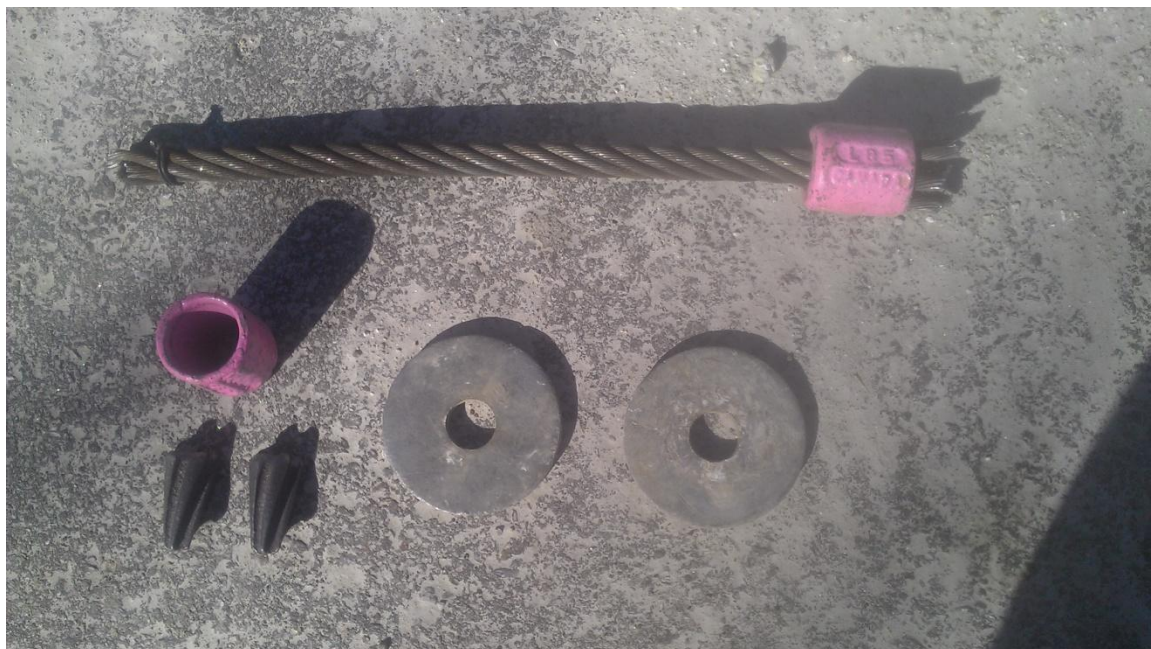
Figure 4.6 Cable Bolt Components
